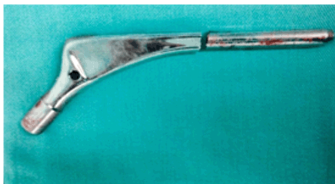
Figure 6: Detail of the fractured implant.
