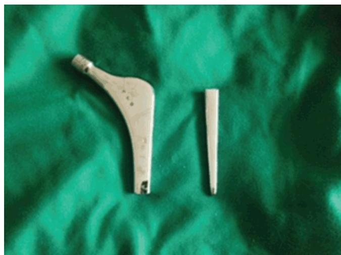
Figure 3: Fractured implant (TIFF).
